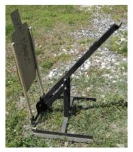
Manufacture: NEVCO Targets Quantity: 2 Stored: Conex 2 Action: The target will expose itself once or can remain in the upright position. Setup Notes: Weights can be adjusted for different rates of exposure.
