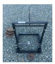
Device: Bobber Target Manufacture: Range Master Steel Quantity: 1 Stored: Conex 2 Action: Target moves up and down once or can swing up and down several times. Setup Notes: Adjust main weights and counterbalance weight to obtain desired results.
