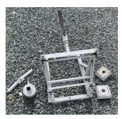
**Device:** Up/Down Target **Quantity:** 1 **Stored:** Conex 2 **Action:** Target moves up and down once or can swing up and down several times. **Setup Nature:** The kettle weight is for repetitive up and down. Even weight a
