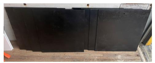
Device: 18x24 AR Plates Quantity: 8 Stored: Conex 2 Action: Used to protect props or decrease the view of targets. Setup Notes: Height of target depends on size of post used. This rated at A36 steel.
