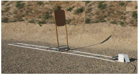
Device: Attack Target Manufacture: MGM Targets Quantity: 1 Stored: Conex 2 Action: The target travels down the track in less than 2 seconds. Setup Notes: Target may be mounted in the trolley parallel or perpendicular to the track. For set-up assistance contact the equipment manager. Do not place any weights on the trolley because it will cause damage to the driving mechanism.
