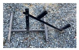
**Device:** Drop Out Target **Quantity:** 2 **Stored:** Conex 2 **Action**: Target falls to the side. **Setup Notes:** The swing arm can be adjusted to different heights.
