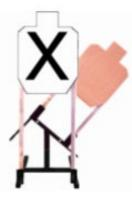
Device: Out and Back Target Stand Manufacture: GT Target Stands Quantity: 2 Stored: Conex 2 Action: The target swings out and then back. It can be set to just swing out. Setup Notes: Adjust weights to change the rate of movement.
