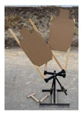
Device: Double Swinger Manufacture: NEVCO Targets Quantity: 1 Stored: Conex 2 Action: The targets swing back and forth. Setup Notes: Weights can be adjusted on targets to vary the rate of swing. There is a custom post designed for the prop, shown in picture.
