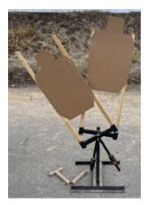
Device: Double Swinger Manufacture: NEVCO Targets Quantity: 1 Stored: Conex 2 Action: The targets swing back and forth. Setup Notes: Weights can be adjusted on targets to vary the rate of swing. There is a custom post designed for the prop, shown in picture.
