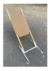
Device: <u>Cardboard Target Stand 45°</u> <u>Manufacture: MGM Targets</u>, (Home made) <u>Quantity</u>: 3 MGM, (5 homemade wooden versions) <u>Stored</u>: Conex 2
