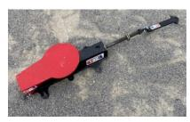
Device: "Bigfoot" Stomp Plate Manufacture: USA Targets Quantity: 2 Stored: Conex 2 Action: Device will pull cable when stepped on. Setup Notes: Pins on sides will come out from time to time.
